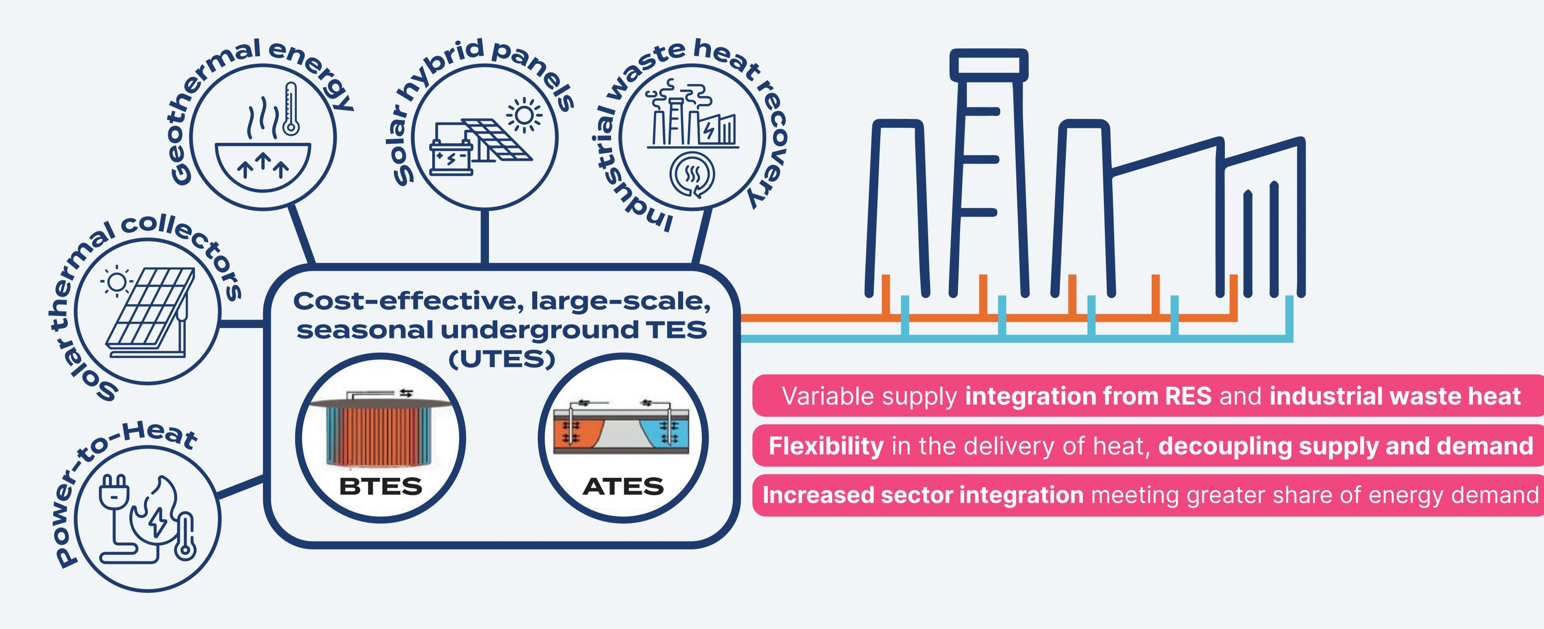
Two large-scale underground thermal energy storage units and four replication cases, using renewable energy sources, waste heat and innovative technologies to decarbonised district heating networks and heat supply
