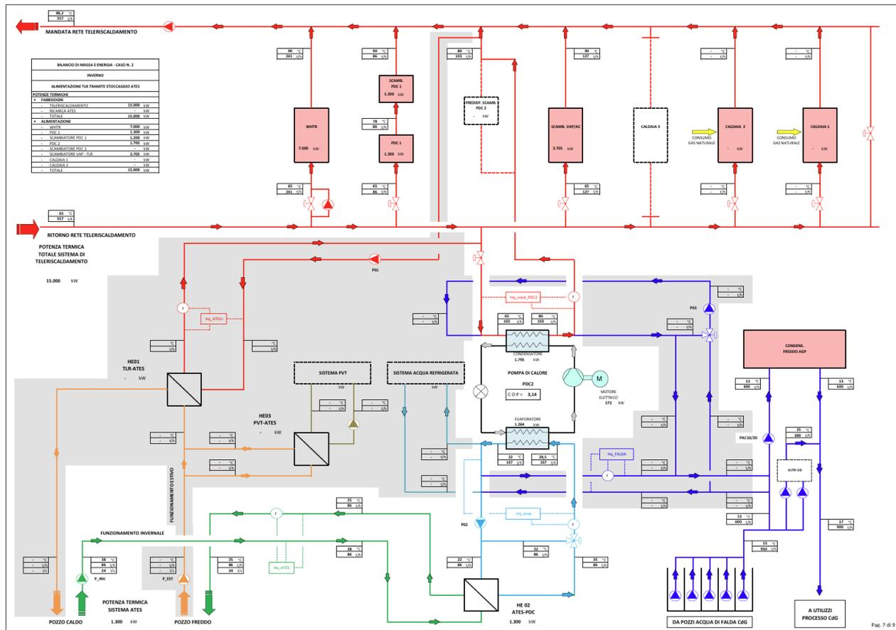
Figure 41. Preliminary conceptual flow scheme for the ATEs system operating in discharging mode during the wintertime at the Riva del Garda demo site.
