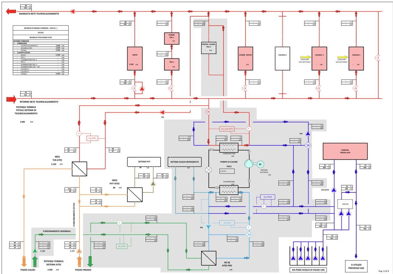
Figure 40. Preliminary conceptual flow scheme for the ATEs system operating in charging mode during the summertime at the Riva del Garda demo site.
