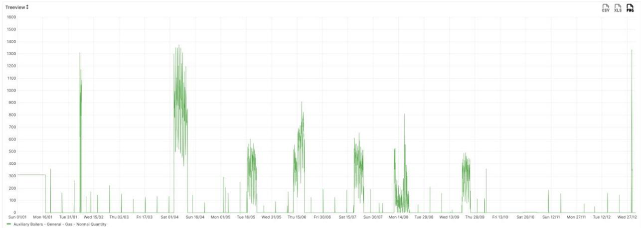
Figure 25. Hourly natural gas consumption profile for 2023 of the auxiliary boilers at the AGP plant. The vertical axis represents natural gas consumption in Sm<sup>3</sup>, while the horizontal axis corresponds to the date.
