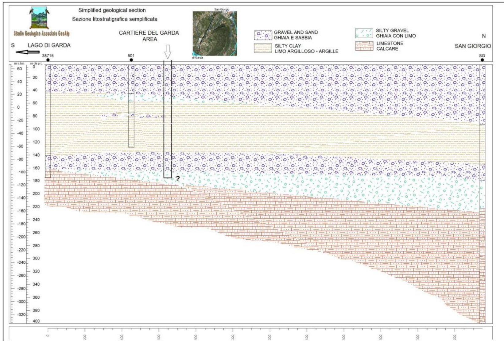
Figure 8. Interpreted stratigraphic section of the subsurface geology between San Giorgio di Arco and Lake Garda.
