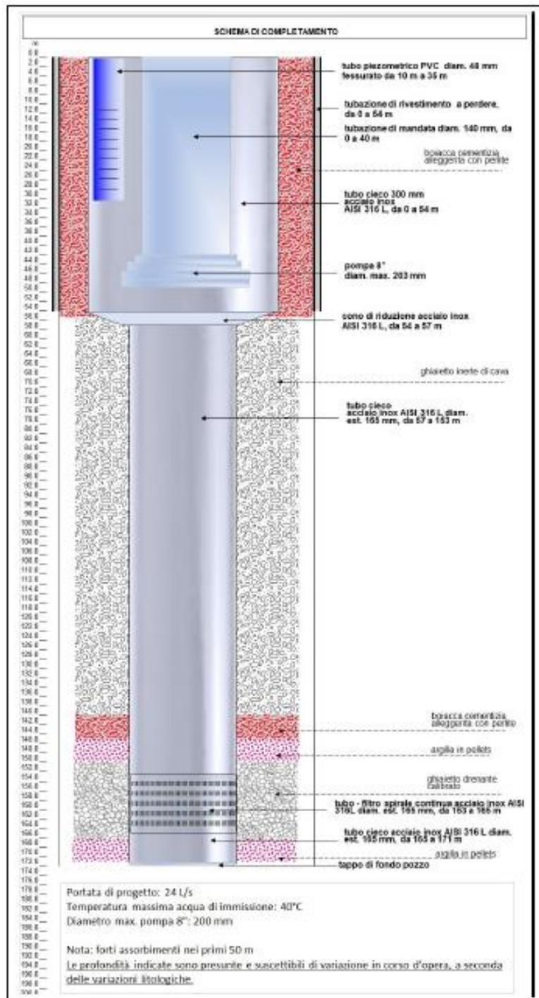
Figure 30. Preliminary construction scheme for the ATES wells.
