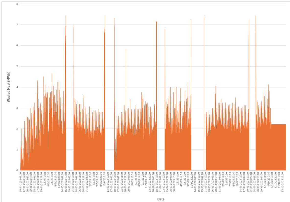
Figure 20. Hourly profile for wasted heat from AGP plant in Riva del Garda in 2023.
