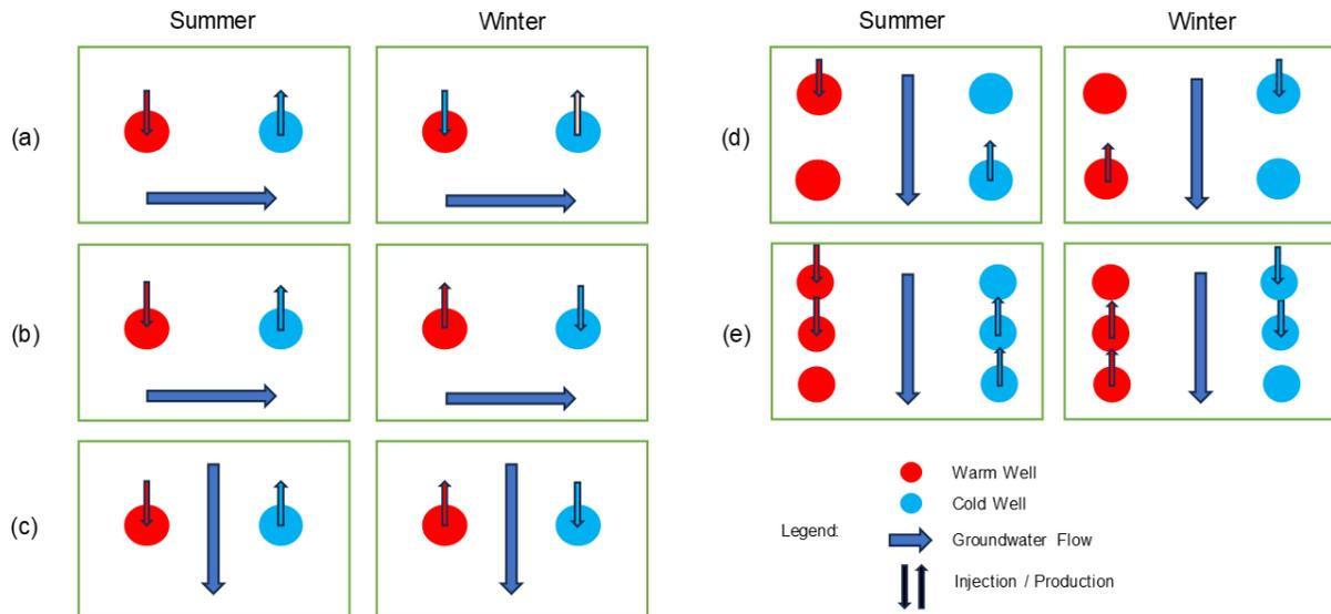
Figure 28. Different well placement settings, showing: (a) Initial two-well setting adopted to this project; (b) two-well setting in the direction of groundwater flow with low efficiency; (c) two-well setting for recovery maximization; (d) four-well setting; and (e) six-well setting.
