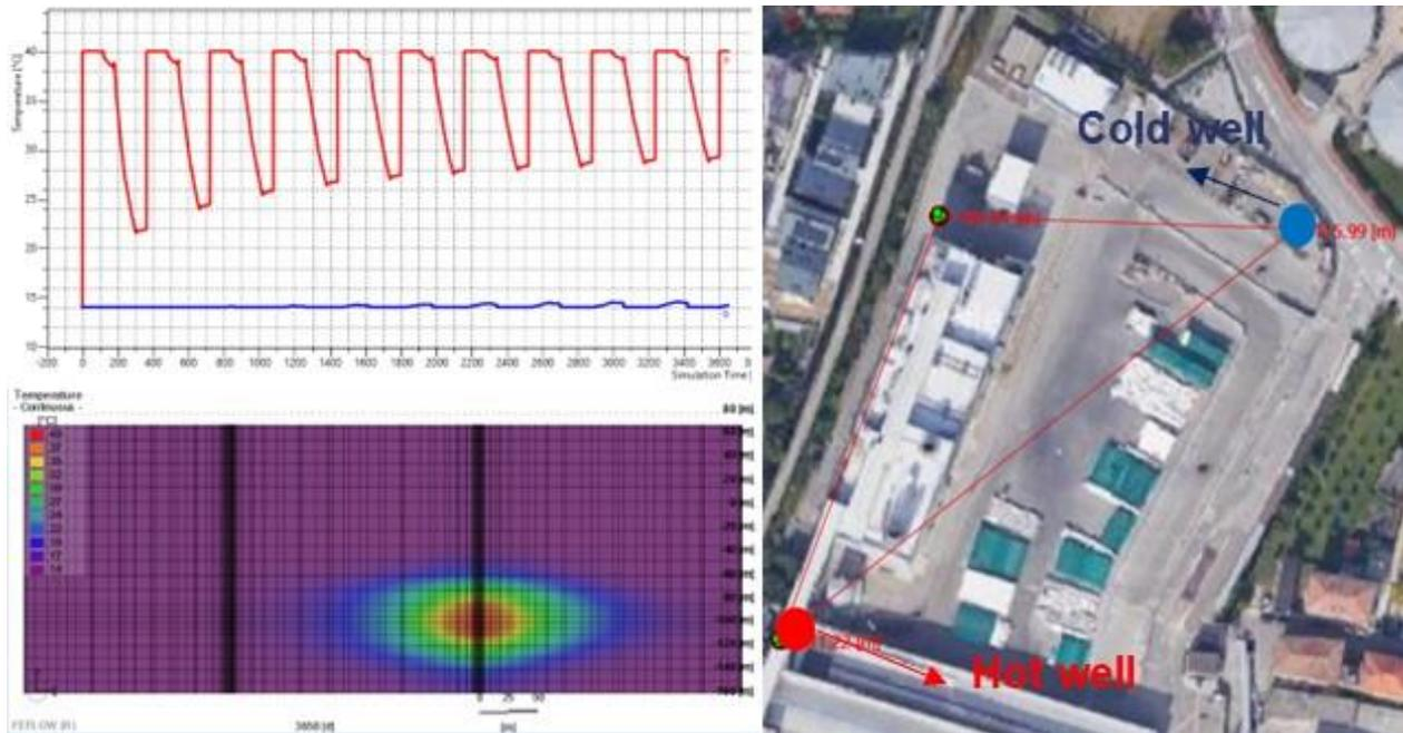
Figure 39. Simulation results for the ATEs system with a mass flow rate of 24 l/s over a duration of 10 years at the Riva del Garda Demo site.
