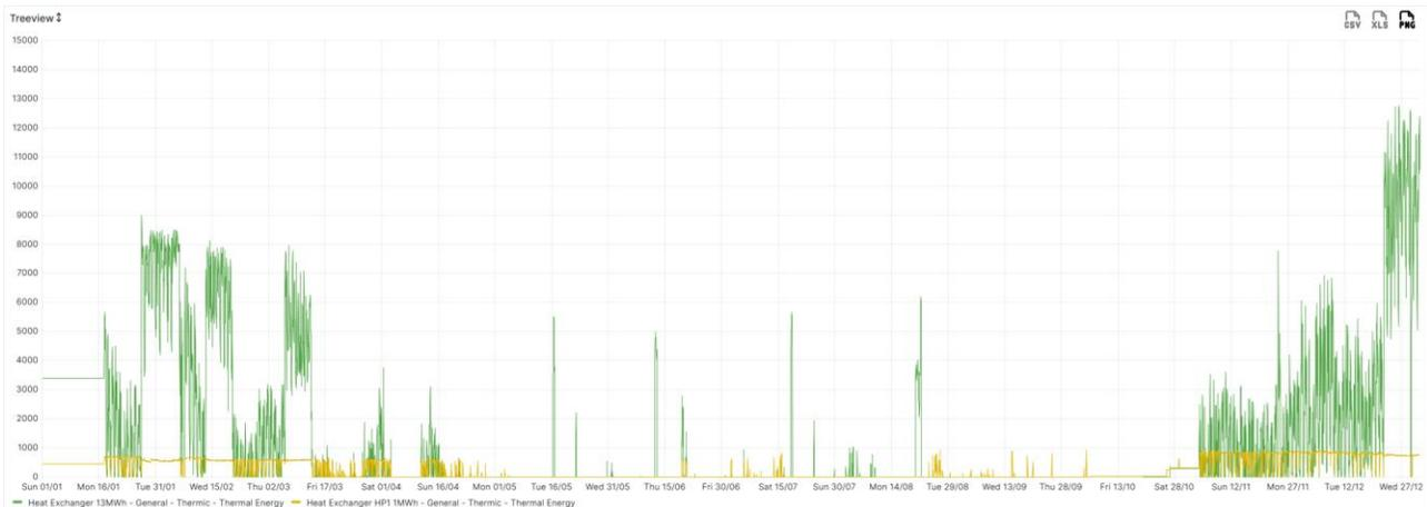
Figure 22. Hourly profile for 2023 of the current heat exchangers at the AGP plant, illustrating the delivery thermal energy for heat exchangers 1 (green line) and 2 (yellow line). The vertical axis represents energy in kWh, while the horizontal axis corresponds to the date.
