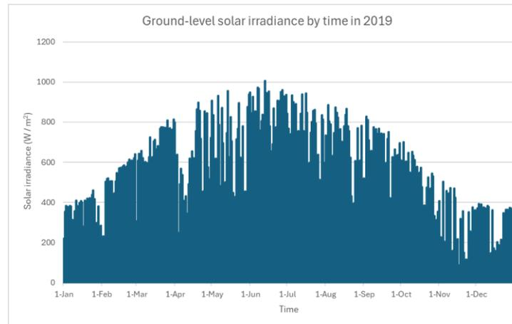
Figure 4. Surface-level incident shortwave radiation flux, considering cloud cover and aerosols in Riva del Garda for 2019 [Renewables.ninja].
