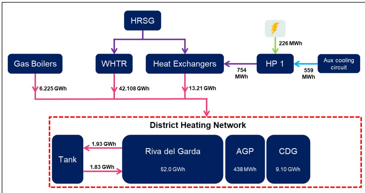
Figure 17. A simple schematic illustrating the energy flows supplying the district heating network in Riva del Garda for the year 2023.
