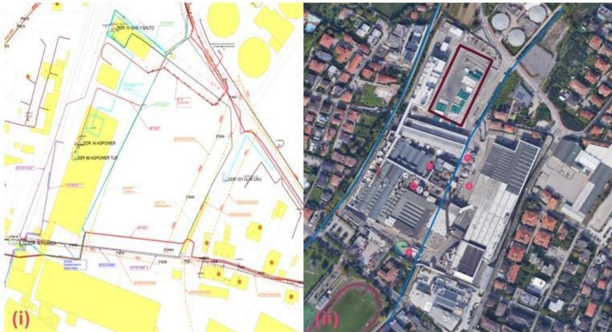
Figure 38. (i) Underground infrastructure owned by AGS and located at the Riva del Garda Demo site; (ii) Position of existing groundwater wells (pink points), rivers (blue line), and commuting area (red rectangle).
