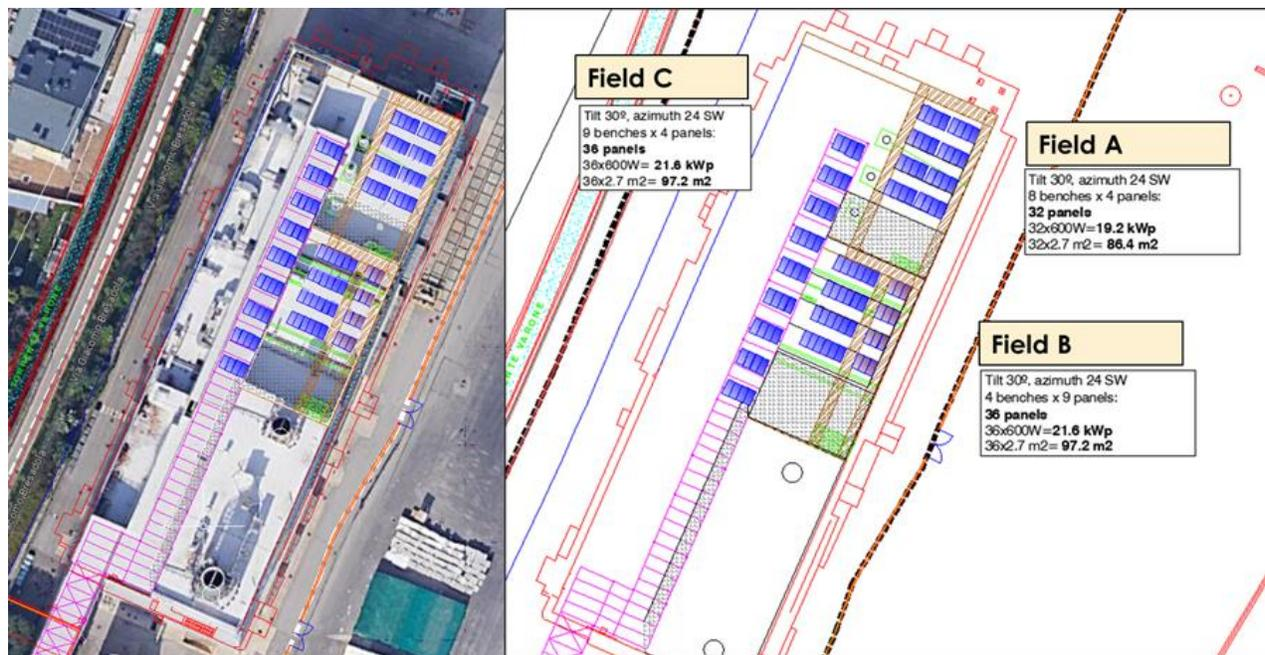
Figure 44. PVT panels fourth layout proposed by ENDEF for Riva del Garda demo site.
