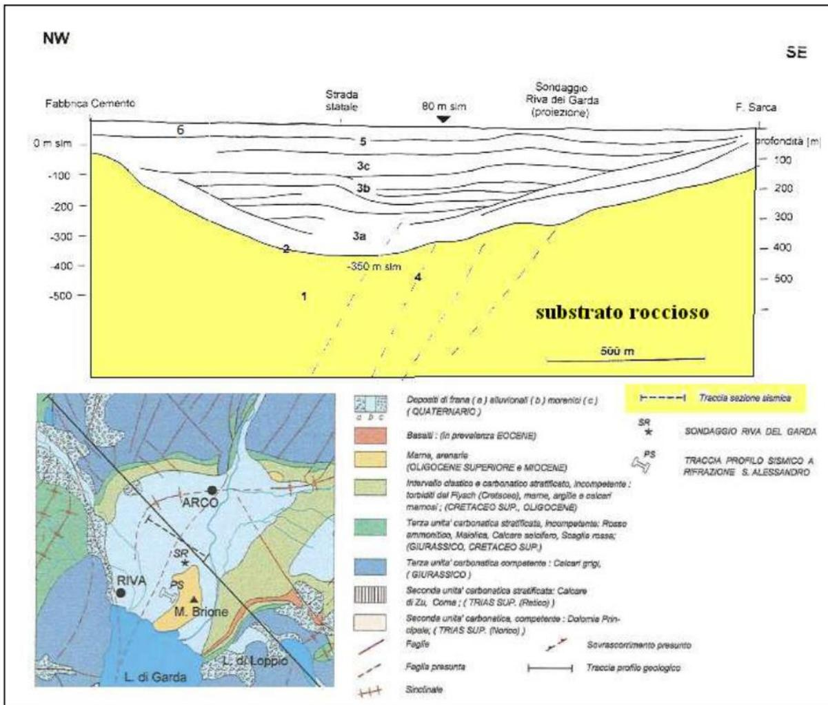
Figure 6. Seismic section (from Felber et al., 1998, with modifications). Profile interpretation legend: 1: bedrock; 2: top of bedrock; 3a: glacial deposits; 3b: cemented sands; 3c: fluvial deposits; 4: faults; 5: lacustrine facies deposits; 6: fluvial and torrential alluvium. The trace of the seismic section is shaded in the geological diagram.
