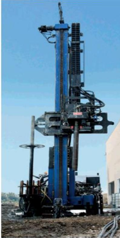
Figure 32. Drilling machine (Joy 5) previously developed by HYDRA in the projects Cheap-GSHPs and GEO4CIVHIC.
