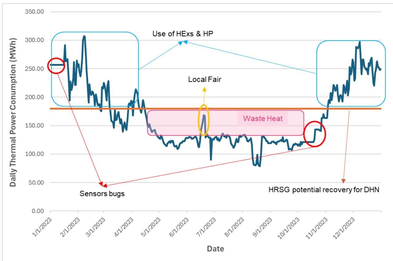
Figure 15. Daily supply profile for district heating network, highlighting the HRSG potential, available excess heat during the summertime, and the utilization of heat pump and heat exchangers to meet the peak demand during wintertime.
