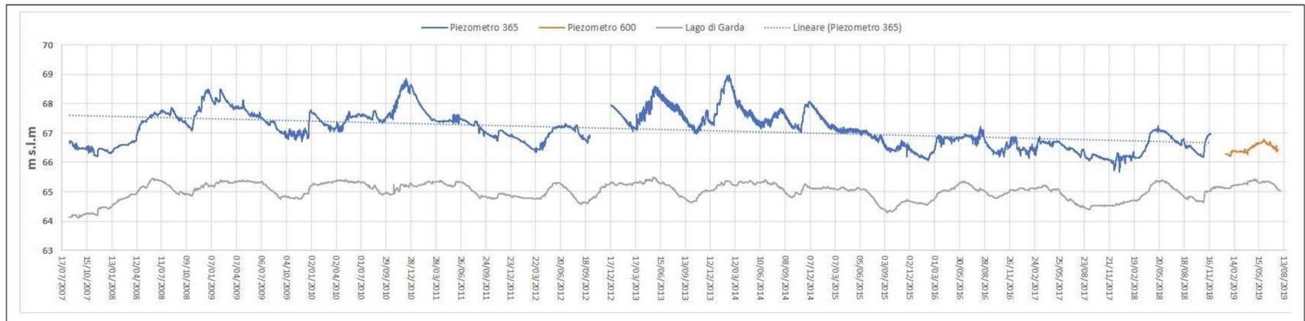
Figure 11. Water table level data from piezometer located in Riva del Garda at PAT purifier from 2007 to 2018 and comparison with the levels in the lake Garda.
