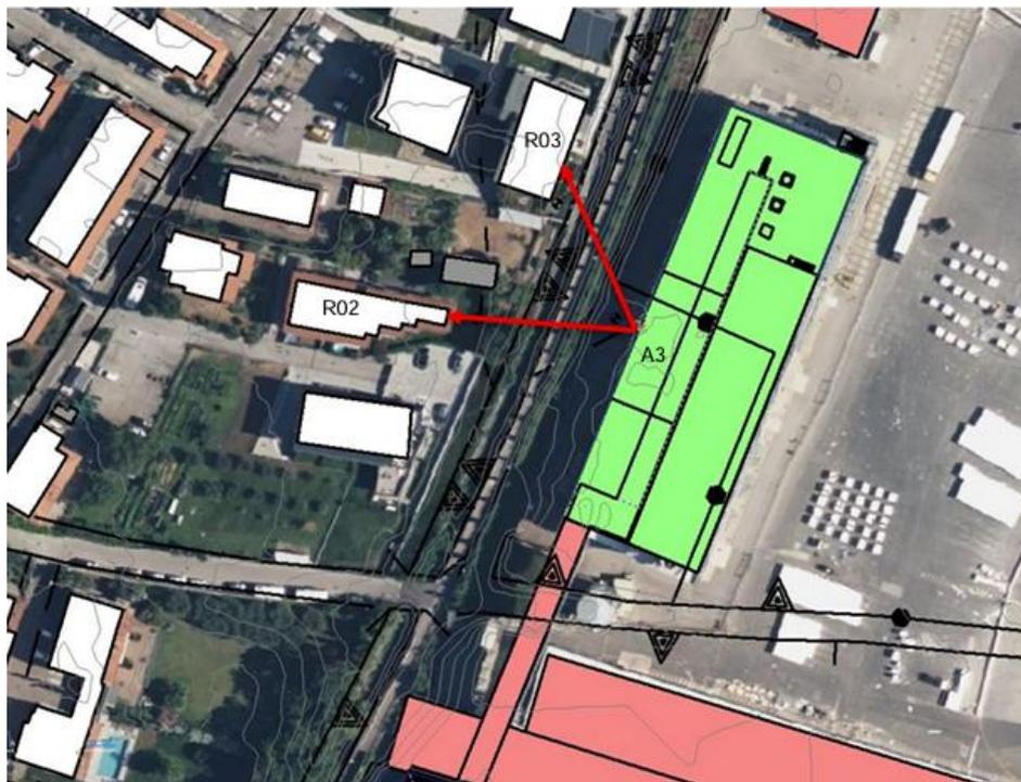
Figure 42. Area of interest with the identification of receptors involved in the acoustic study.
