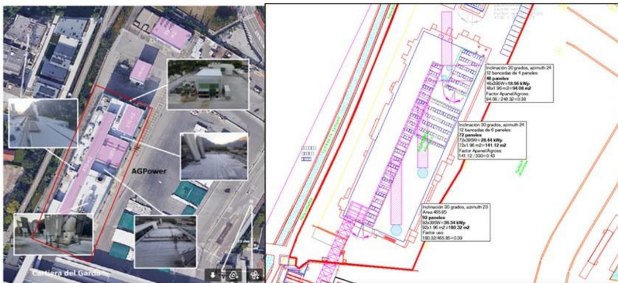
Figure 34. Schematic of the initially proposed locations and the corresponding number of panels planned for installation at the Riva del Garda Demo site.
