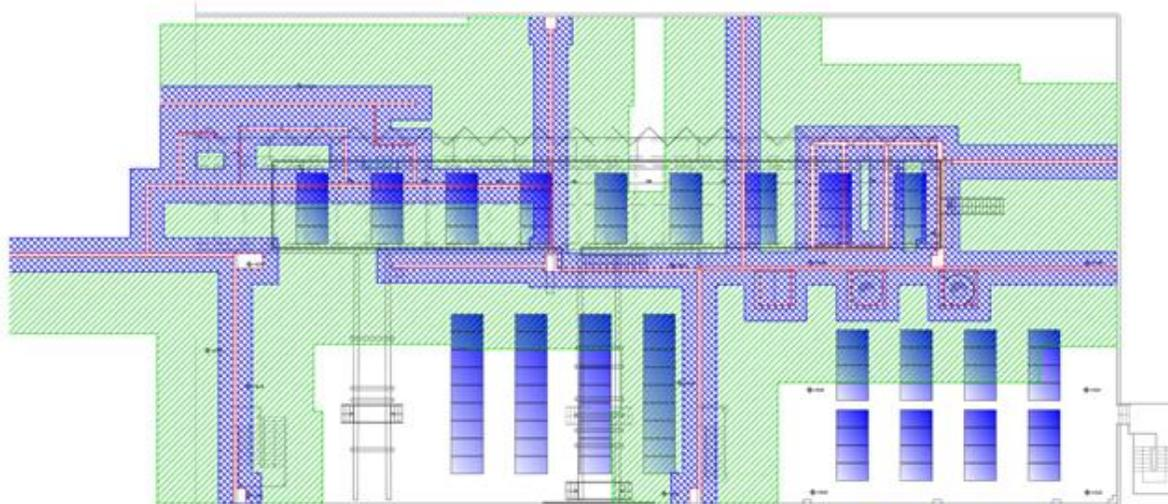
Figure 45. AGP roof layout showing buffer areas.
