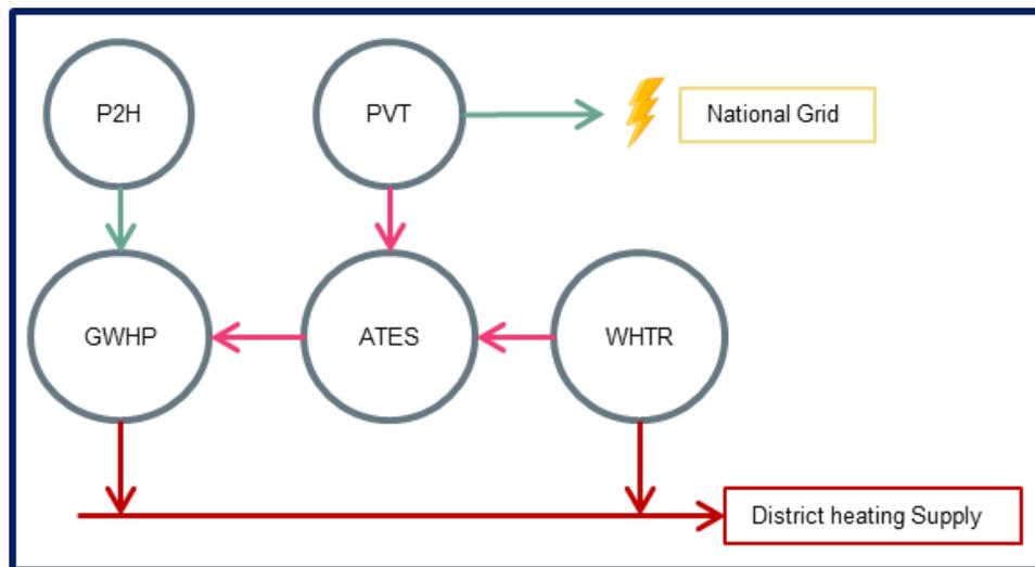
Figure 26. General conceptual flow scheme planned for the integration of technologies at the Riva del Garda demo site.
