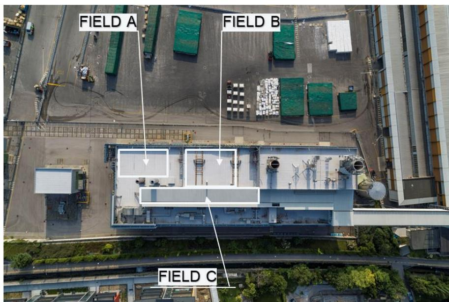
Figure 35. Top view of Alto Garda power, indicating the proposed locations for installing the PVT panels at the Riva del Garda Demo site.
