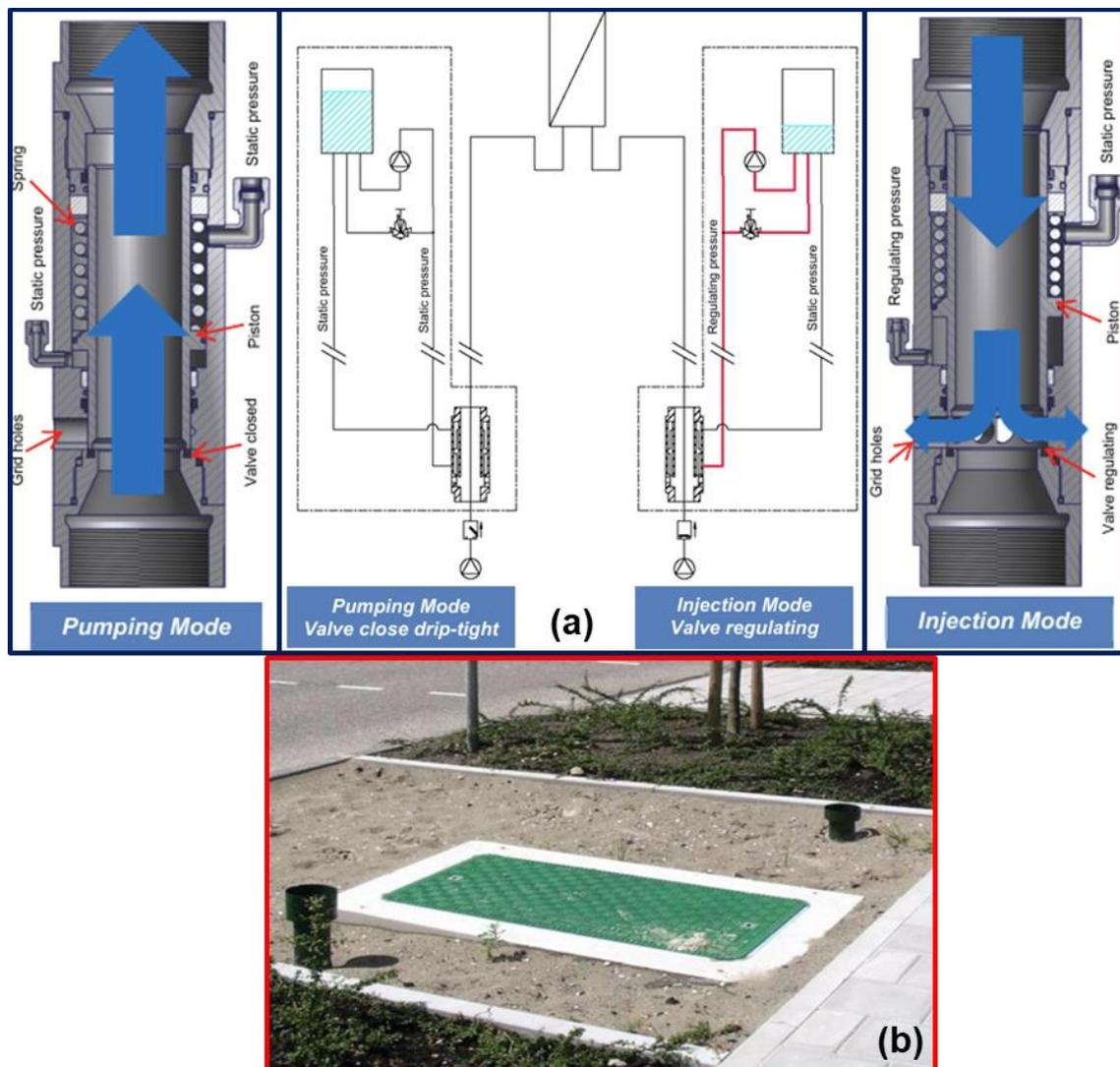
Figure 31. (a) Simple schematic of the injection valves proposed for installation in the ATEs system; (b) Underground Finish type of well housing proposed for construction.
