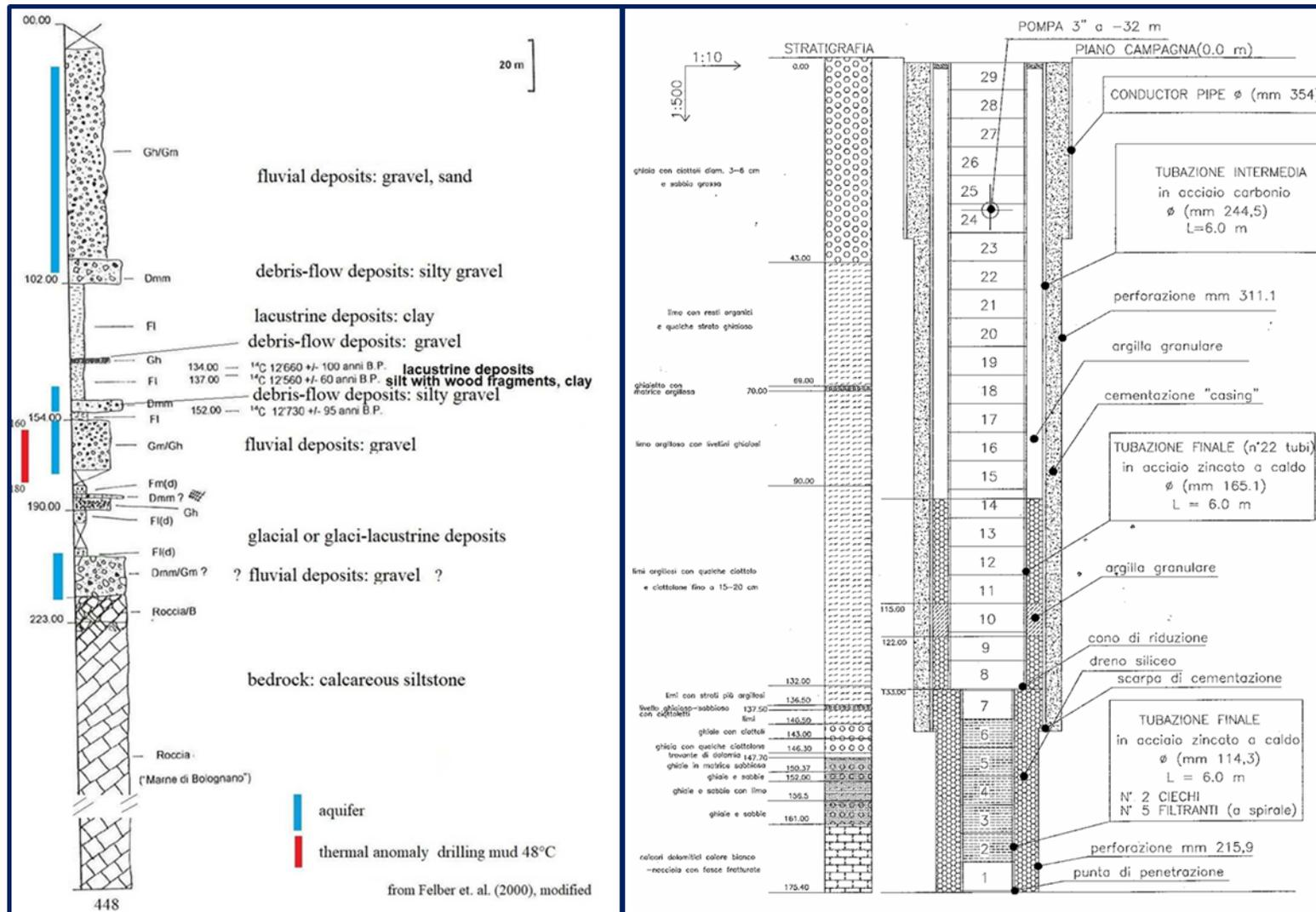
Figure 7. Stratigraphy of the deep exploratory well in San Giorgio di Arco with sedimentological interpretation (left); construction scheme with stratigraphy of deep well called Fonte Brione drilled at Park Hotel Du Lac (right).
