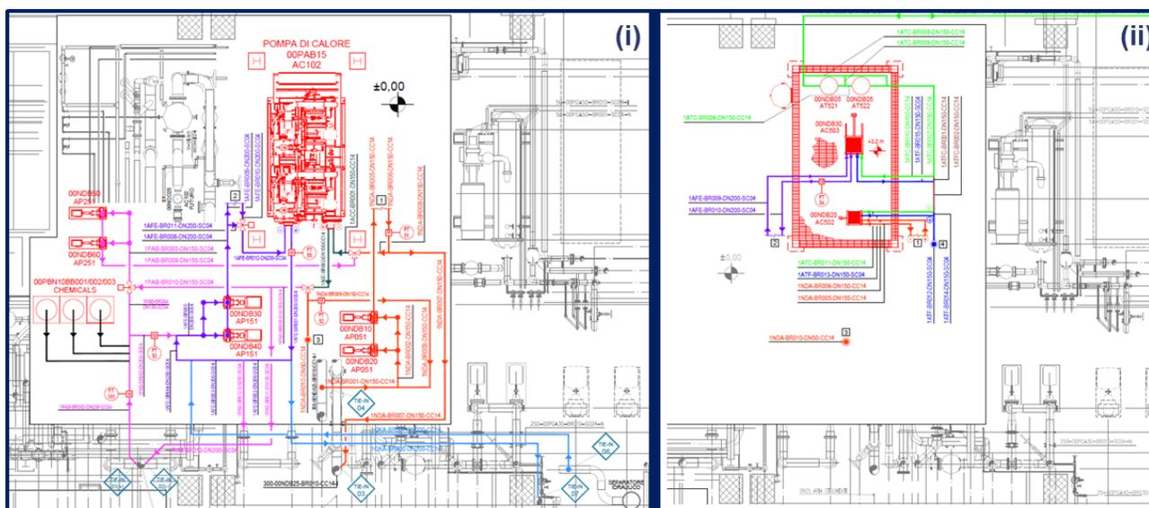
Figure 43. Planned area for the new heat pump in the room with the current pipeline at the AGP plant; (i) +0.0 m elevation; (ii) +3.2 m elevation.
