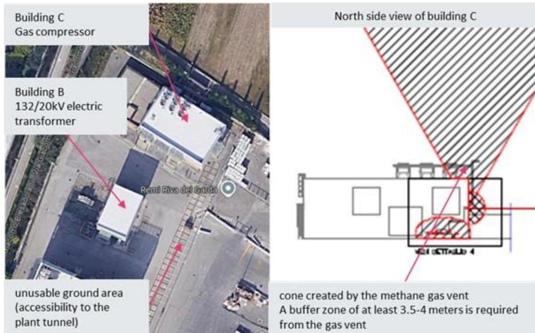
Figure 36. Alternative positions for PVT panels installation at the Riva del Garda Demo site.
