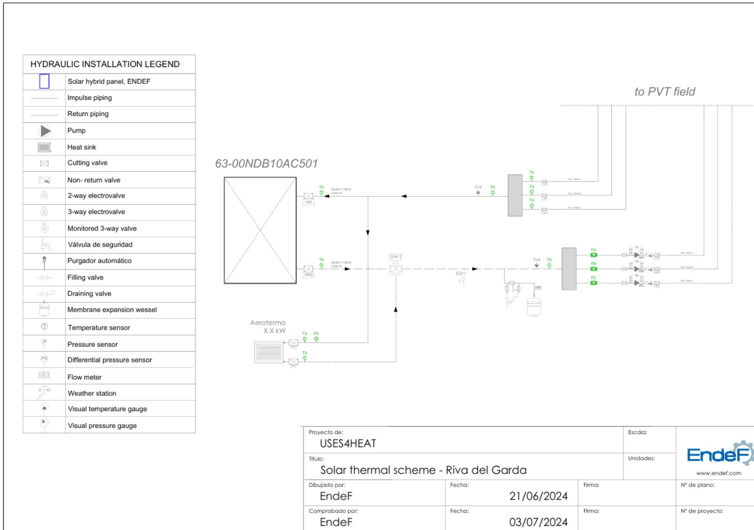
Figure 37. P&ID for the integration of PVT panels with the heat exchanger connected to the ATEs system.
